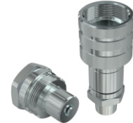
PVVM Screw to connect couplings for high pressure, ISO 14540 interchange, poppet valve (WP upto 1000 Bar)
