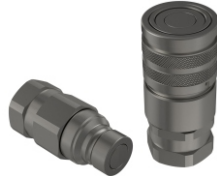
FFH Flat face couplings, ISO 16028 interchange, 350 Bar series.
